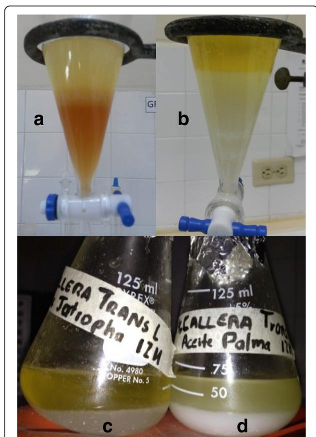
**Fig. 1** Enzymatic biodiesel produced with Jatropha and palm oil. **a** The alkaline-catalyzed biodiesel produces a reddish-brown glycerol phase. **b** Enzymatic biodiesel catalyzed by CA produced a cleaner (white) glycerol phase. **c** Jatropha biodiesel catalyzed by TL. **d** Palm biodiesel produced with TL enzymatic catalyst. One advantage of enzymatic biodiesel over alkaline catalyzed biodiesel is a cleaner, higher-quality glycerine by-product
