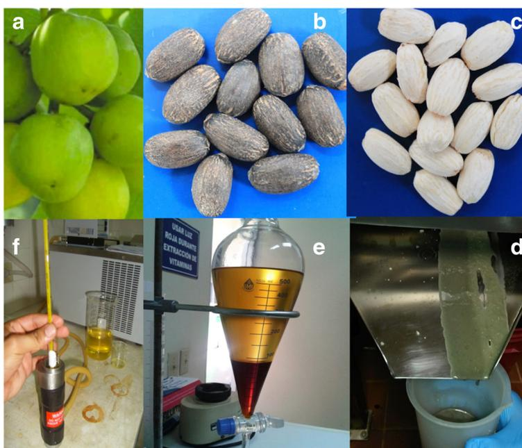
**Fig. 3** Production of *Jatropha* biodiesel. **a** Fruits of *Jatropha*, Cabo Verde variety. **b** Mature seeds of *Jatropha*. **c** Dehusked seeds of *Jatropha*. **d** Mechanical *Jatropha* oil extraction with expeller. **e** *Jatropha* biodiesel at phase separation step. Top phase is biodiesel and bottom phase is glycerol. **f** Cloud point measurement of *Jatropha* biodiesel
