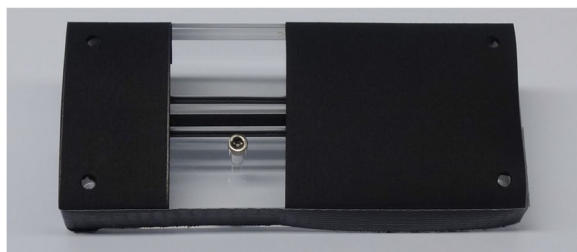
Fig. 7 Experimental Setup for Continuous Excitation. The channel has been covered with black paper to define the starting point of isomerization. Flow from left to right
